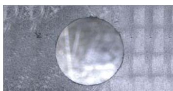
Fewer burrs on workpieces
