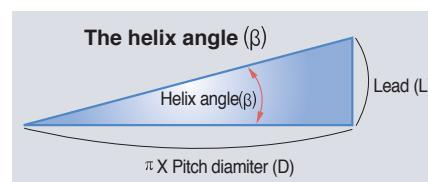
For a straight thread, where the lead of the thread and the pitch diameter circle circumference form a right angled triangle, the helix angle is the angle opposite of the lead
