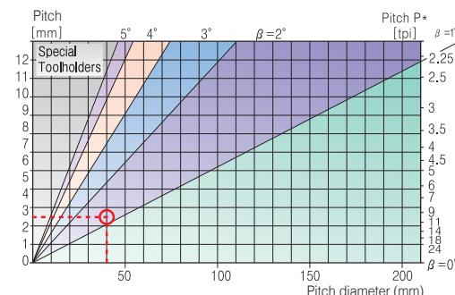
From the table, using a pitch of 2.5 mm(10 tpi) and a workpiece diameter of 40mm (.157"), we find the helix angle to be 1.5°
