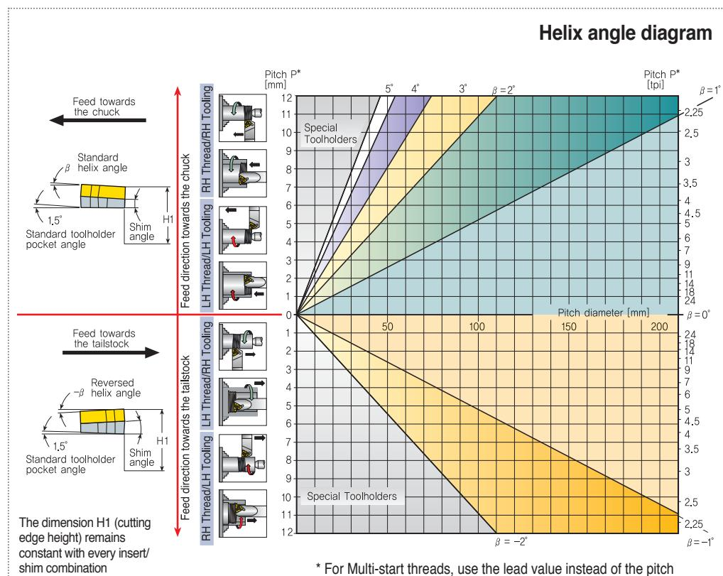
\* For Multi-start threads, use the lead value instead of the pitch
