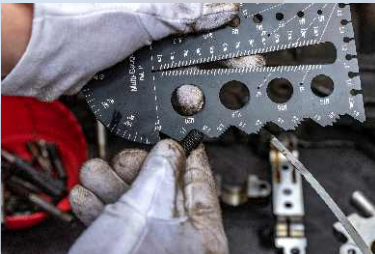
Pitch Size Measure the Thread
