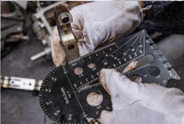
Gage Leg Quick-Check Perpendicularity
